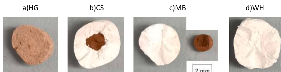
Fig. 3. Image of the synthesized MAC beads: a) Homogeneous (HG), b) Core-shell (CS), c) Mixed bed (MB). The pellet of zeolite 13 \times used in experiments with resistive wall heating (WH) is also shown.
