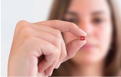
Figure 2 The CUBE mXTEND™ antenna booster from Fractus Antennas has a volume of 5 mm 3 .
