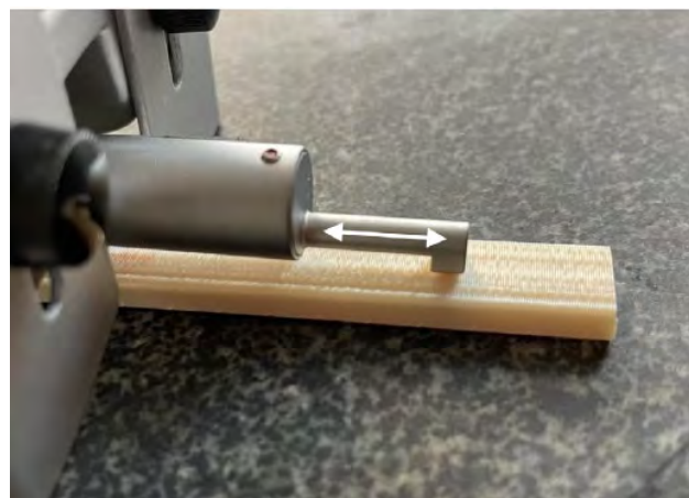
Figure 3: Photograph of a ZX (printed upright) specimen showing the evaluated face and the direction of the surface roughness measurements (indicated by a white arrow).
