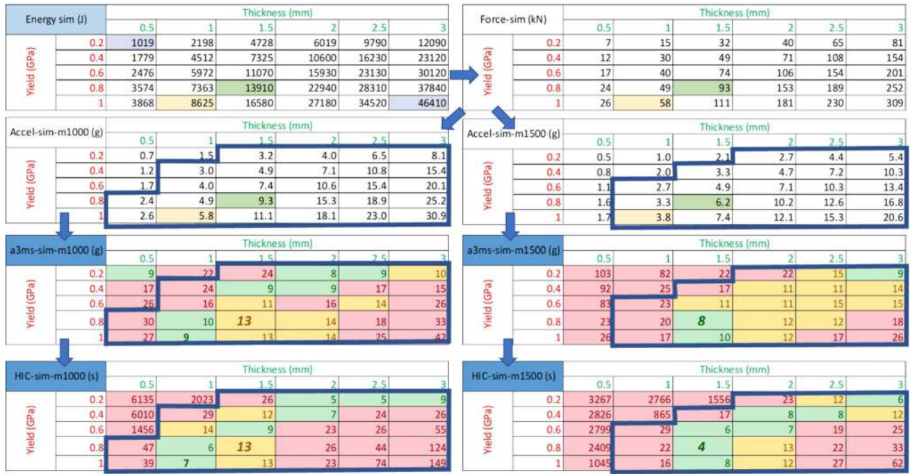
Fig. 7 Energy and force from compression used to estimate best deformation element to fulfil acceleration a3ms and HIC injury criteria for 1000 and 1500 kg
