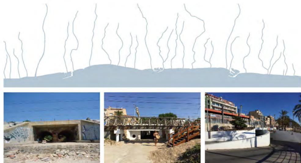
Figure 6. Transversal permeability studies the connectivity between the inland area and the beach, following the streams which cross infrastructures through underground passages (Source: authors' own).
