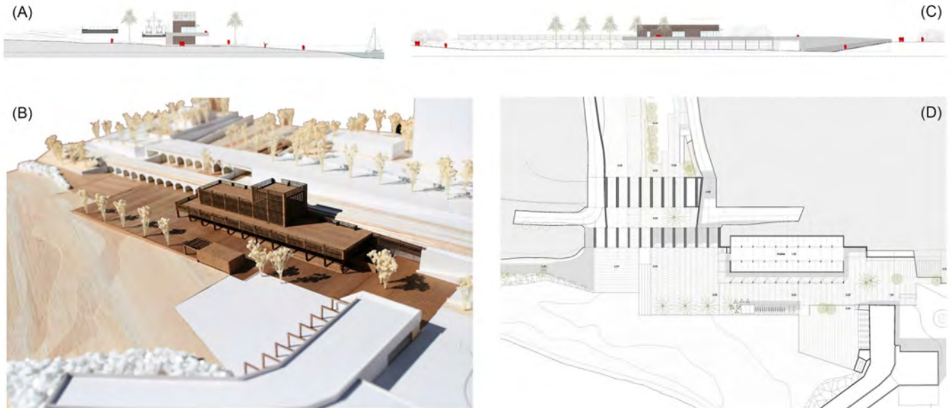
Figure 12. Urban and architectural project for the case study of the stream mouth in Llavanes (Source: authors' own). (A) Transversal section of the underground passages. (B) Model picture of prefabricated constructions. (C) General elevation of the maritime façade. (D) General floorplan with green treatment of the stream, floodable squares and light-weight constructions for local services and the railway station.
