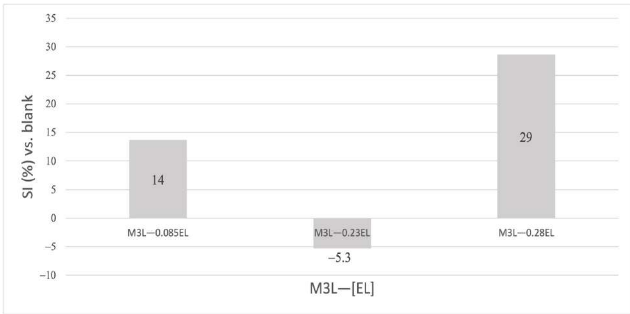
Figure 11. Mean swelling indexes (%) for EL membranes normalized vs. blank membranes with EL at 0.085, 0.23, and 0.28% in 3L.
