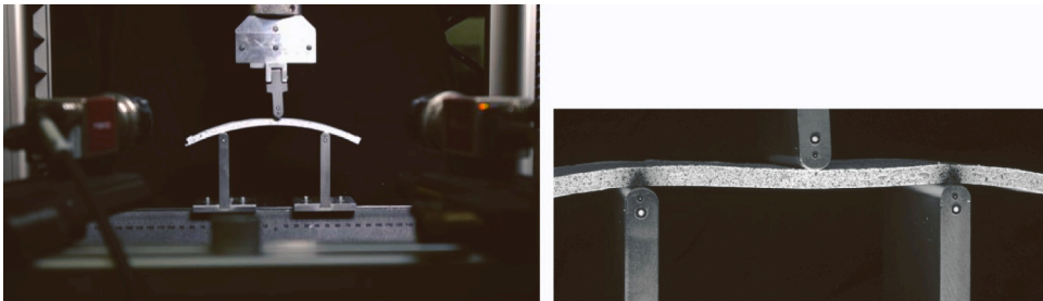
Fig. 10. Digital Image Correlation setup used during the three-point bending test of curved samples.
