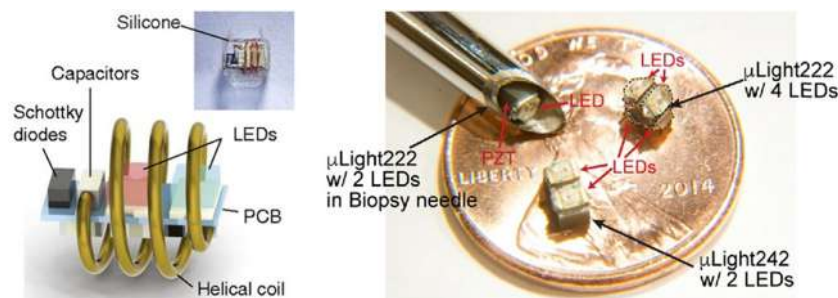
Figure 10: Examples of implantable wireless light sources powered by an external radiofrequency source (left) and by ultrasound emitter (right). Images adapted from refs [77] and [78], respectively.
