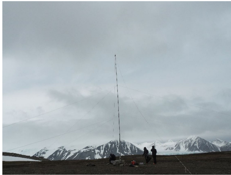
Fig. 22 Rocky Glacier remote node installation. Installation of second remote node in the Antarctica scenario. This node was situated 5 km away from the central node
