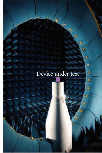
FIGURE 6: Anechoic chamber having a gate with 31 probes to electrically measure the radiation in one plane radiated by the device under test. The device under test is rotated so as to have the full 3D data.
