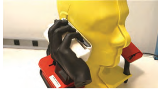
FIGURE 5: Over-the-air phone testing in the talk position, including the phantom hand.
