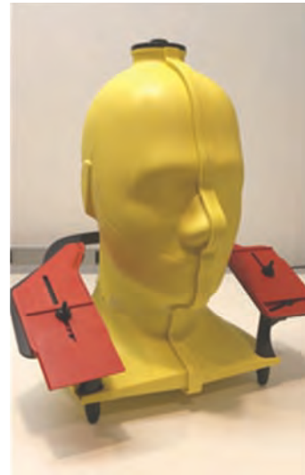
FIGURE 2: A model of the specific anthropomorphic mannequin (SAM) head.
