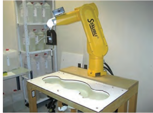
FIGURE 4: SAR measurement system. The wireless handheld device radiating RF power is attached to a phantom cheek. A probe measures the electrical field generated by the device inside a phantom filled with liquids emulating the human tissue at the frequencies of interest.
