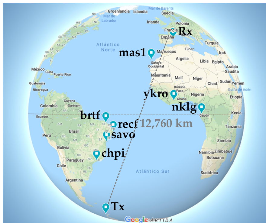
Figure 1. Geographical link characteristics. The transmitter (Tx) is located in the Spanish Antarctic Station (SAS), Livingston Island, and the receiver (Rx) is placed in Cambrils, Spain. Furthermore, the Global Navigation Satellite System (GNSS) receivers of the International GNSS System (IGS) used to detect the irregularities associated with the equatorial plasma bubbles (EPB) are shown: mas1 ( 27.61^{\circ}\text{N} , 15.63^{\circ}\text{W} ); nklg ( 0.35^{\circ}\text{N} , 9.67^{\circ}\text{E} ); ykro ( 6.83^{\circ}\text{N} , 5.24^{\circ}\text{W} ); brtf ( 3.85^{\circ}\text{S} , 38.43^{\circ}\text{W} ); chpi ( 22.55^{\circ}\text{S} , 44.98^{\circ}\text{W} ); recf ( 8.00^{\circ}\text{S} , 34.95^{\circ}\text{W} ); and savo ( 12.86^{\circ}\text{S} , 38.43^{\circ}\text{W} ).
