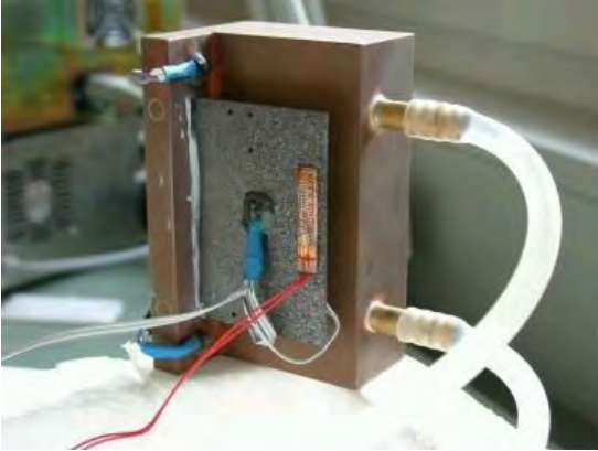
Figure 3.47: Photograph of the setup used to measure thermal conductivities.
