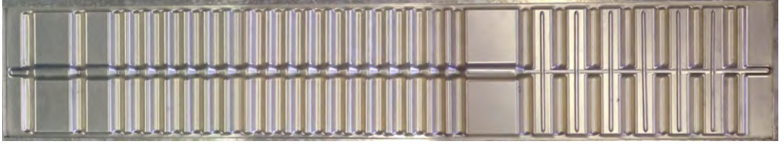
Figure 3.4: Top foil of the detector vacuum box, made from 0.3 mm thick AlMg3. The structure is 120 cm long, the width is 25 cm.
