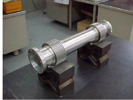
Figure 2.6: Prototype bellows machined at CERN.
