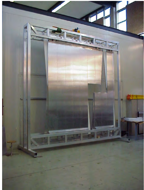
Figure 5.17: Mockup for the study of station assembly.
