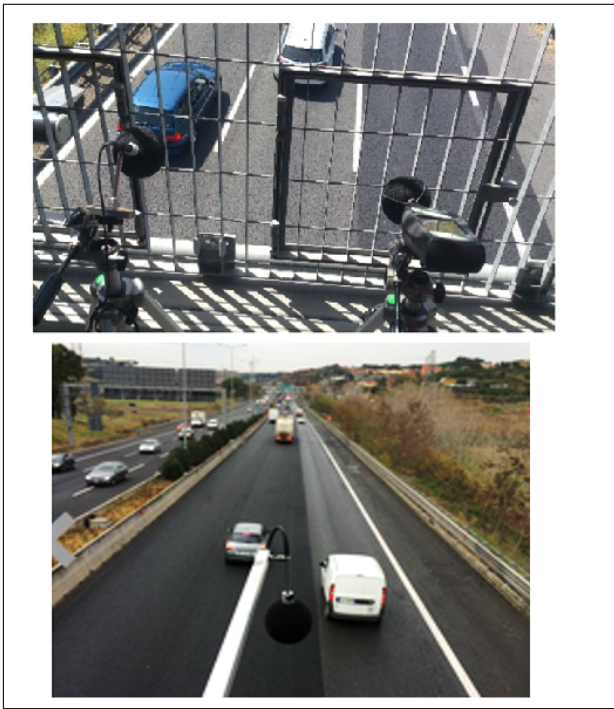
Figure 1. Example of the sensors positioning during the recording campaign (top) and in the definitive installation (bottom) within the WASN.
