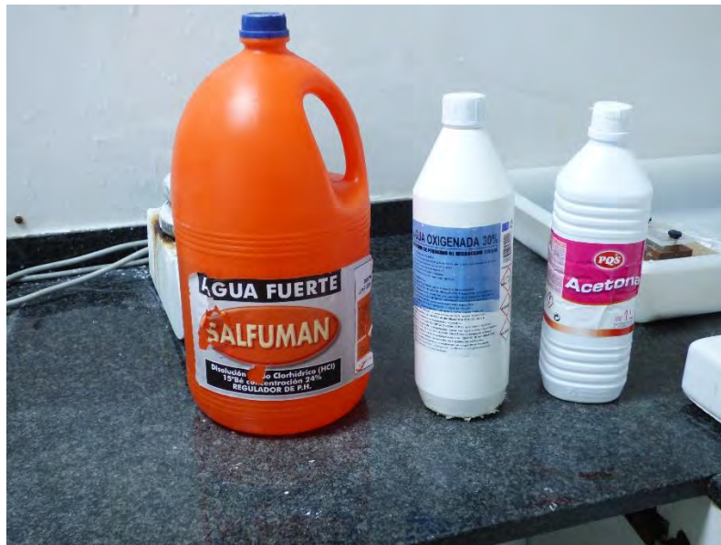
Figure 52 From left to right, the components used to create the PCB in the chemical lab: Hydrochloric acid, Hydrogen peroxide, Acetone.
