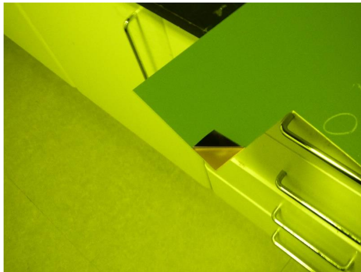
Figure 51 Piece of FR4 substrate used for the Prototyping making off, without a piece of protective fiber, which shows the top layer copper.
