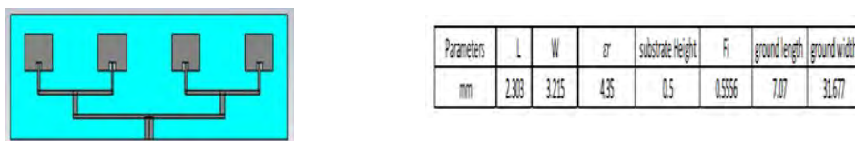
Figure 31. 4-element Microstrip Patch antenna array and its parameters
