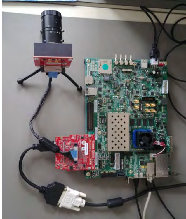
Figure 10: Set up with the new board ZCU106. The connections are the same as with the previous board.
