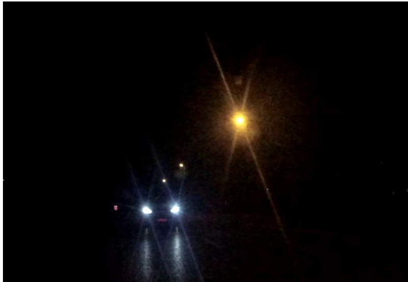
Figure 29: Sample of low-light situation. The light sources and its reflections are the only visible thing. Besides the two frontal lights of a vehicle, three street lights are visible. The artifacts that appear in this picture won't be present in a CMS as the cameras and preprocessing used in those systems reduce the presence of those.
