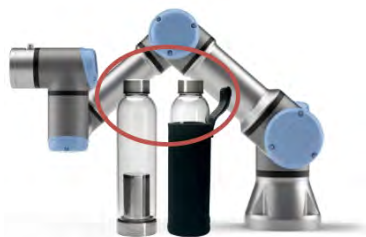
Figure 37: Example of collision between the UR3 arm and some bottles.
