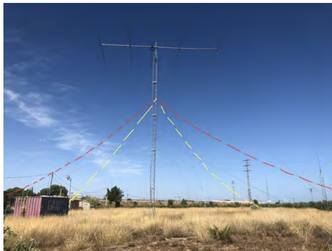
Figure 3.5: Reception antennas in Cambrils. Two inverted vee antennas made of a flat copper, positioned orthogonally, tunned at 5.4MHz and located in Sant Josep's of La Salle. 7
