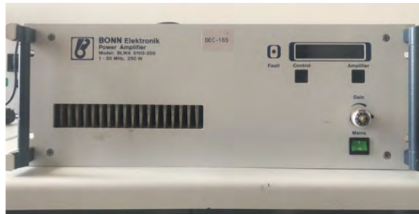
Figure 3.8: HF Power Amplifier, Model BLWA 0103-250 used in the transmitter 7
