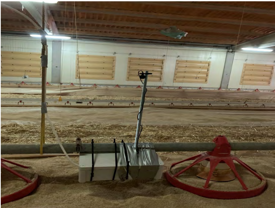
FIGURE 2.2: Acoustic recording prototype for deployment in a Poultry Farm Source: [34]
