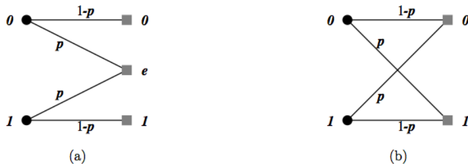
Figure 4.1: Two examples of channels: (a) The Binary Erasure Channel (BEC) with erasure probability p , and (b) The Binary Symmetric Channel (BSC) with error probability p .
