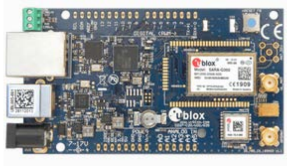
Figura 6. U-Blox C027 Application board.
