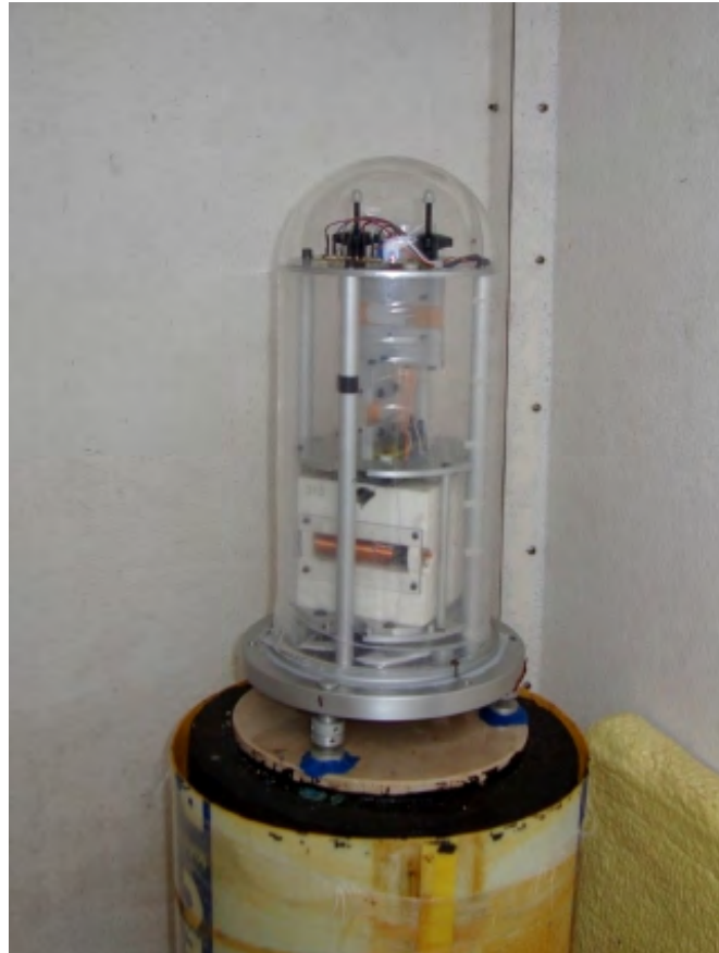
Figure 4. The three-axis automatic fluxgate magnetometer was added in 2008. More details about the sensor can be found in [9].
