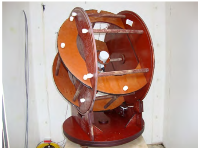
Figure 3. \delta D/\delta I vector magnetometer deployed at the ASJI with the two perpendicular pairs of Helmholtz coils and the proton magnetometer allowing one to measure the variations of D/I. More details about the sensor can be found in [9].
