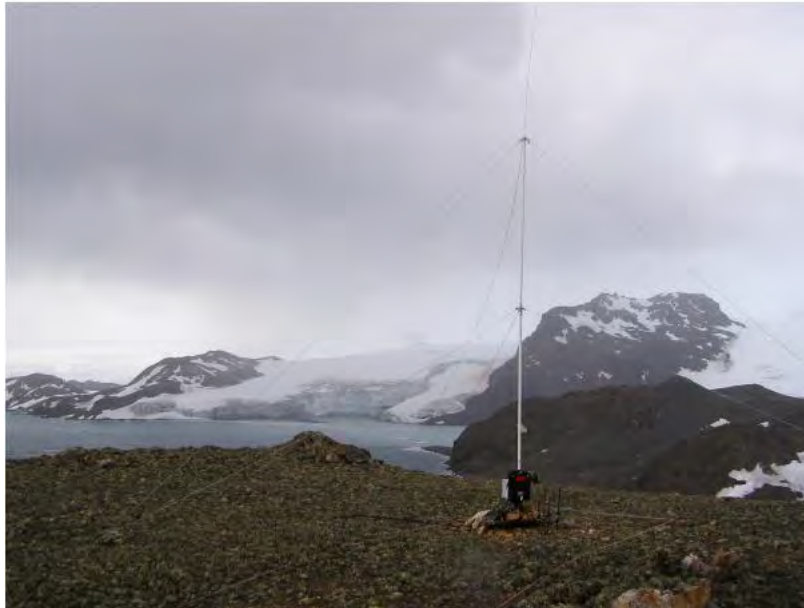
Figure 7. The antenna of the oblique ionosonde transmitter at the ASJI.
