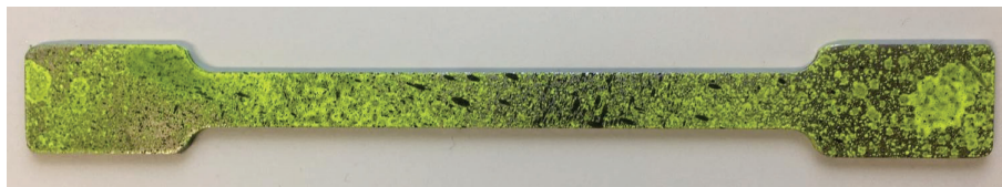
Figure 3. Painted specimen with random pattern for the calculation of deformations.
